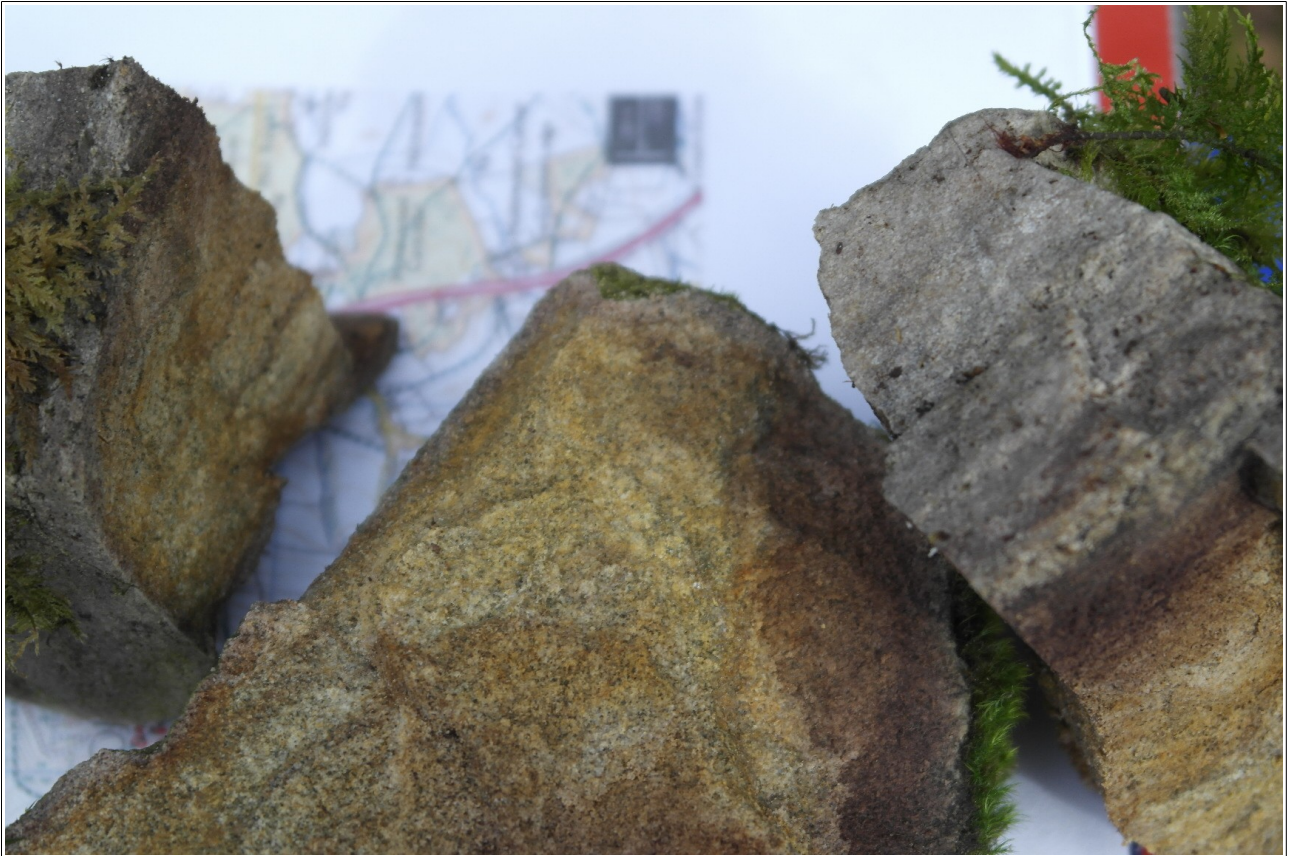
Plate TN1. Highly silicified, fine-grained, competent Lower Greensand sandstone from the Hythe Beds.
